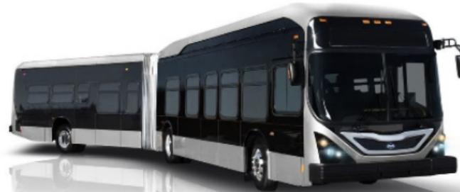
Battery capacity: 652 kWh
